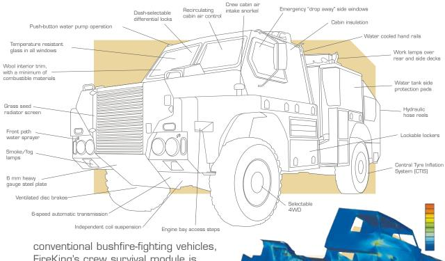
conventional bushfire-fighting vehicles. FireKing's crew survival module is designed to protect the crew of four in emergency conditions.
