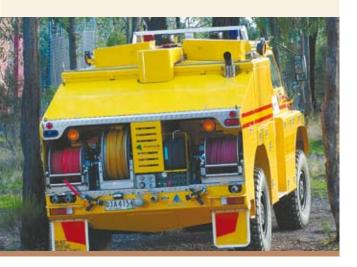
**Main pump** Engine driven through transmission PTO via hydraulic drive constant speed motor
